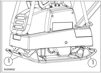
Check the rubber buffers (1) for tears and outbreaks, as well as for secure fit. If they are damaged, replace them immediately.
