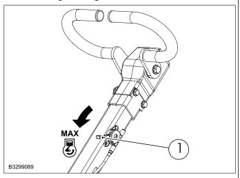
Set the engine speed lever (1) to full load (MAX).
