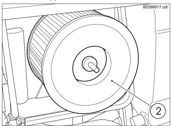
· Carefully remove filter element (2).
