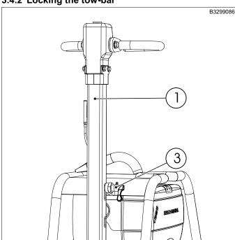
In case of loading and transport the tow-bar (1) has to be locked in an upright position by turning up the locking bolt (3).
