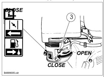
• Move the choke lever (3) to the «CLOSE» position.
