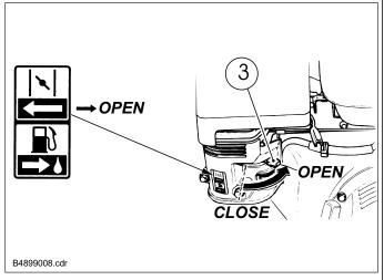
If the choke lever (3) has been moved to the «CLOSED» position to start the engine, gradually move it to the «OPEN» position as the engine warms up.
