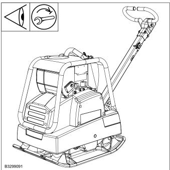
With vibrating devices, it is important to check intermittently the screw connections for tightness. Pay attention to the tightening torque.
