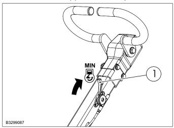
• Set the engine speed lever (1) to MIN.
