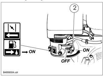
• Move the fuel valve lever (2) to the «ON» position.
