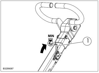
• Set the engine speed lever (1) to the «MIN» position.
