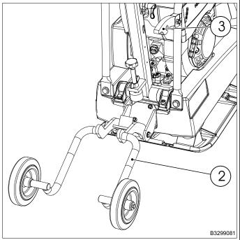
Remove the undercarriage (2) from the mounting bracket (3) and place it on the floor.
