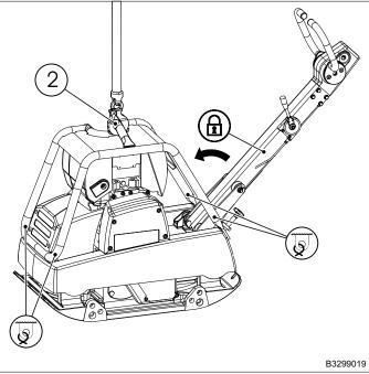
After loading the machine should be lashed in place.
