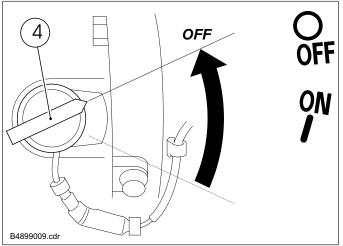
• Turn the engine switch (4) to the «OFF» position.
