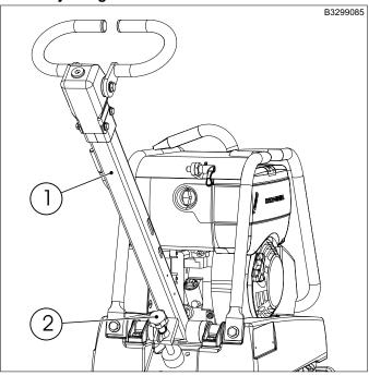
By turning adjustment-screw (2), the tow-bar (1) can be set to any positions so as obtain the best working height on the tow-bar grip.
