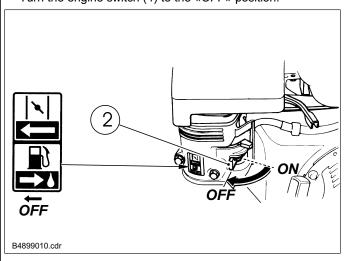
• Turn the fuel valve lever (2) to the «OFF» position.
