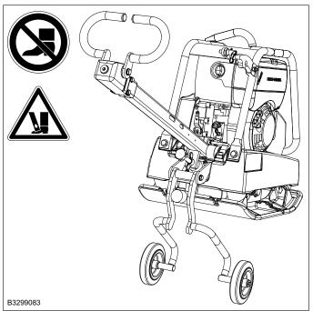
With the towing bar locked in position tip the machine on to the front edge, the undercarriage will swing under the board.
