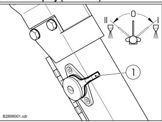
The water spray is switched on and off by the lever (1).
