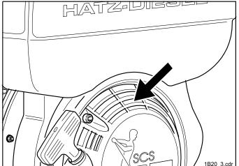
Check intake opening for combustion air and cooling air intakes. Remove coarse ostructions such as leaves, stones and earth.
