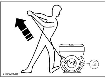
Pull the starting rope with increasing speed, until the motor starts up.
