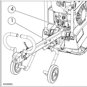
• Position the towing bar (1) horizontally and lock in position (4).
