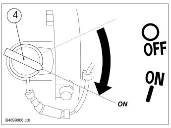
Turn the engine switch (4) to the «ON» position.
