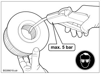
If there is any dry pollution: Blow out the filter cartridge with dry air under pressure (max. 5 bar) from the inside outwards, until no more dust comes out.
