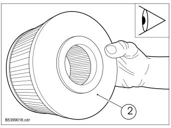
Check filter element (2) for cracks or other damage by holding against the light or using a lamp.
