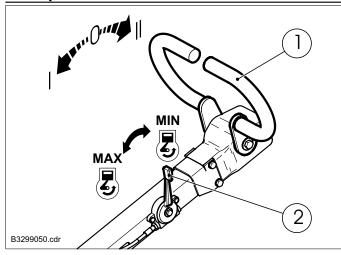
• Set the engine speed lever (2) to full load (MAX).
