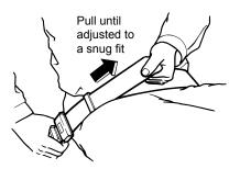
4. Position the seat belt across the lap as low as possible on the hips. Pull the fold-back end of the belt (upper side) until the belt is adjusted to a snug fit.
