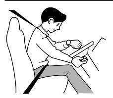
Firmly apply the parking brake. With the accelerator pedal released, turn the starter switch to the "ACC" or "LOCK" position.
