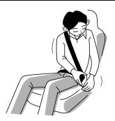
If a vehicle that has seat belts with pretensioner and an SRS airbag system suffers a frontal impact above certain level, seat belts with pretensioner and airbag (including the passenger airbag, if equipped) securely restrain the driver and passenger in their seats and lessen the physical shock to their heads. To prevent the seat belts with pretensioner and airbag themselves from causing life-threatening injuries, be sure to observe the following points:
