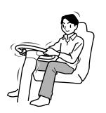
Also check the steering wheel for looseness in mount by moving it back and forth and sideways.
