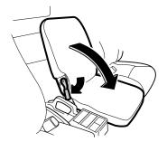
If the center seat is not occupied, fold its seatback forward by using the lever positioned in the side of the center seat.
