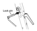
4. Fully lift up the cab, and lock the tilt support while holding the part indicated by the arrow. When it is locked, it makes a "click" sound. Confirm that the lock of tilt support is securely engaged.
