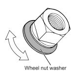
Do not coat with grease (Disc wheel seating surface)
